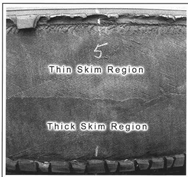
Fig. 10 Rapid tearing region occurring in a field tire tread separation (leading edge flap, left-side tire)
