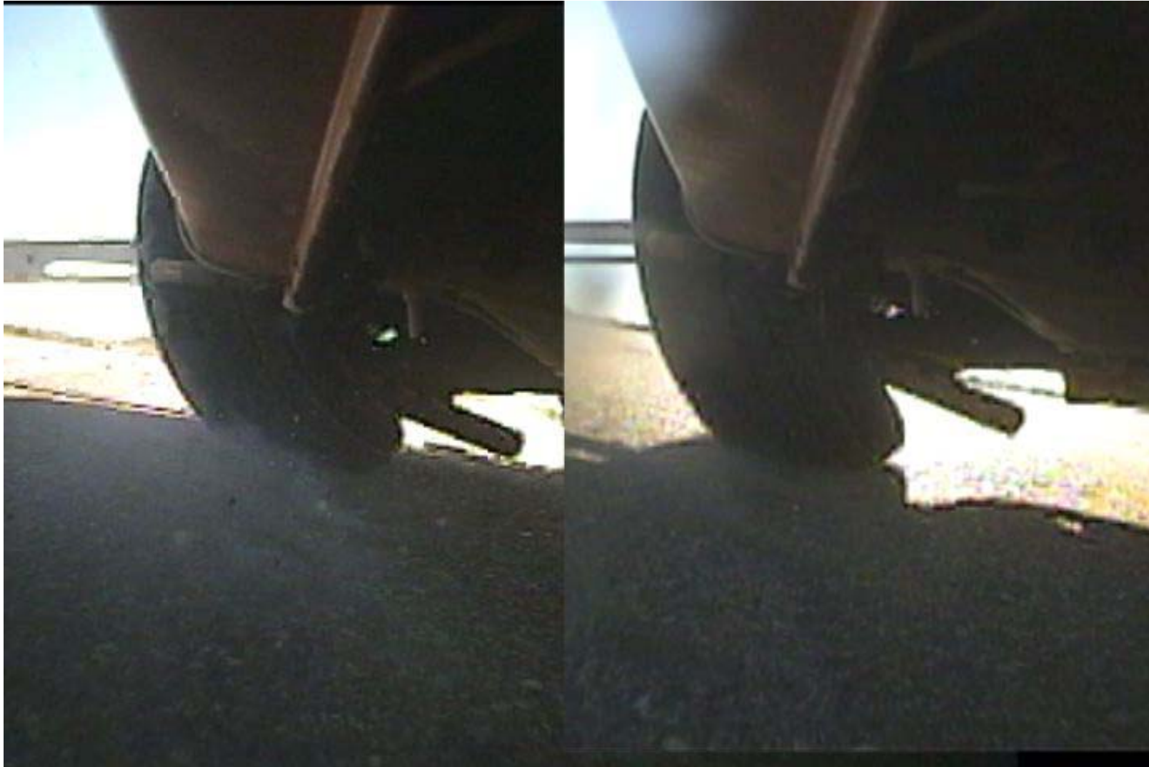
FIGURE 6. Comparison of front tire deformation of P225/75R15 (left) and 31x10.50R15LT (right) at maximum tip-up. Wheels are zero offset in both cases.
