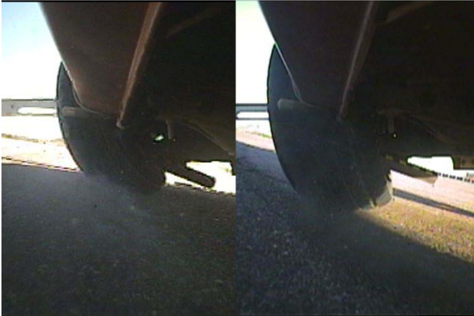
FIGURE 7. Comparison of front tire deformation of P225/75R15 (left) and 285/50R20 (right) at maximum tip-up. Wheels are zero offset on left and -2 mm offset on right.
