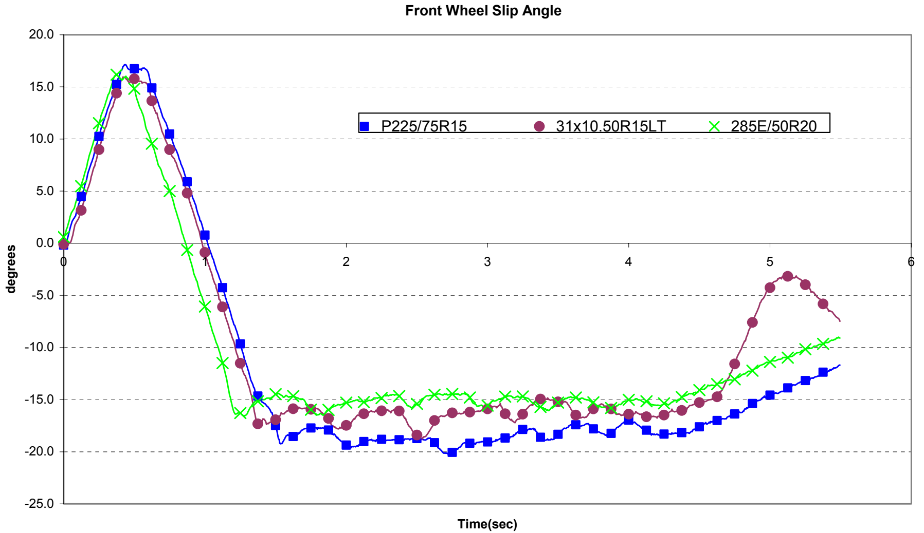
FIGURE 9. Front wheel slip angles for the near-zero wheel offset tests.
