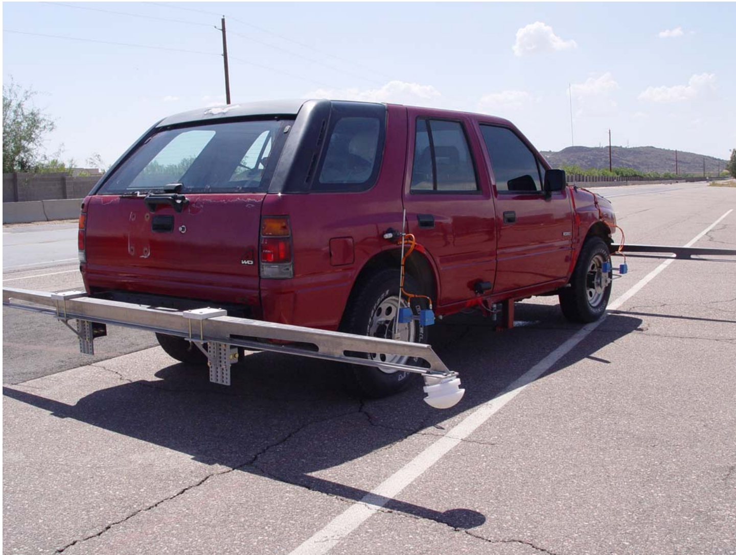
FIGURE 2. Test Vehicle with NHTSA-style outriggers and wheel lift sensors. The steering controller and tire video equipment are specific to this test center.
