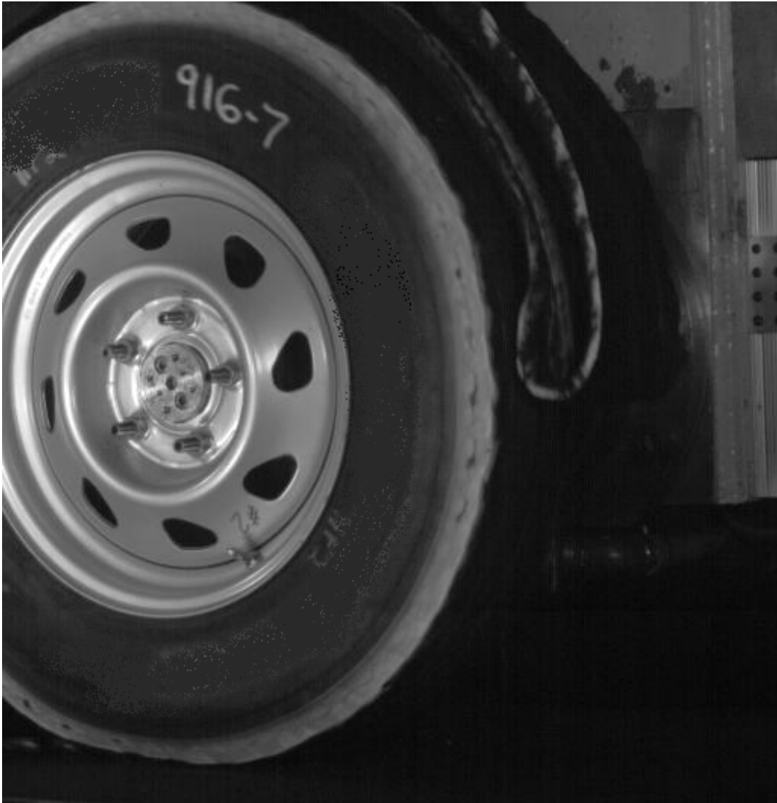
FIG. 1 – Sample video image from high-speed video capture system showing peeling tread and outer steel belt.
